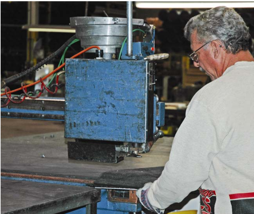
Figure 1 Duro Dyne Rolling Head Pinspotter-Original machine is still a main component in the SMW production line for over 10 years.
