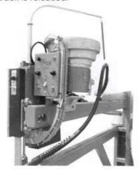
The welding tip glides back and forth along the RH frame eliminating excessive material handling inherent with stationary fastening machines. The five foot throat allows the placement of pins 1½" from each end of a five foot sheet without moving the metal! To convert the RH for fittings, draw the welding tip to the open end of the frame. Slide the quick release pin into position locking the weld tip over the fittings mandril. Remove the handle and connect the footswitch.
