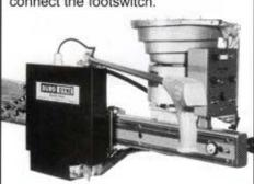
Low voltage (24 volt) electropneumatic circuitry with careful consideration of parts location allows safe and easy access to the rolling assembly components. A pneumatic brake cylinder locks the rolling assembly in position during the weld cycle to ensure a quality weld.
